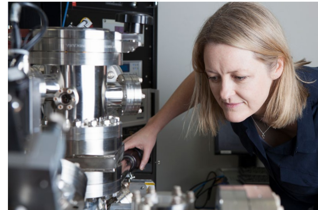
Prof. Julie Cairney using an atom probe. Her team developed cryogenic atom probe tomography, a world-first technique for imaging hydrogen atoms in steel.
