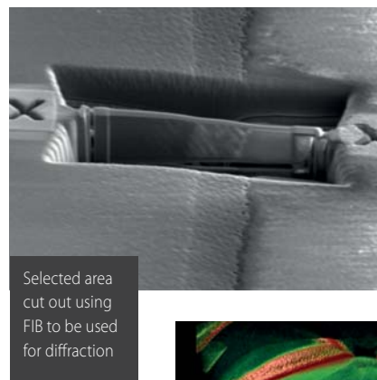
Elemental analysis in SEM showing formation of minerals
