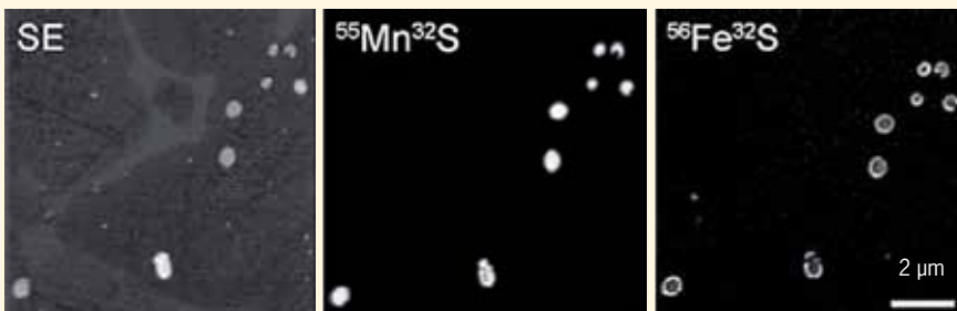
NanoSIMS images of inclusions in a commercial 316-grade stainless steel. Secondary electron image (left), MnS (centre), FeS (right).
