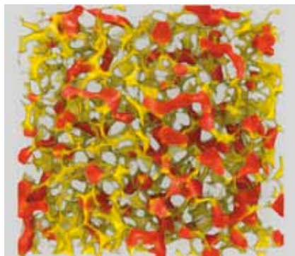
Micro-CT image of residual hydrocarbon saturation in an oil reservoir rock after flooding with water. The rock grains are transparent, showing the water, in yellow, and the residual oil in orange. Filed of view 1.5 mm. Image by Munish Kumar, ANU.
