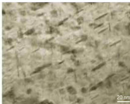
TEM micrographs of the aluminium alloy processed by SPD (left) and by conventional aging (right).
